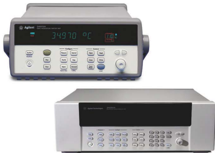
Agilent 34970A & 34980A switch/measure units
